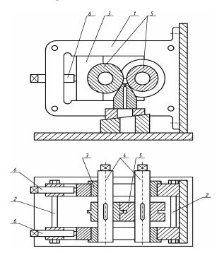
Fig. 2. Laboratory equipment for combined rolling and pressing of aluminum alloys on the basis of rolling mill DUO200
