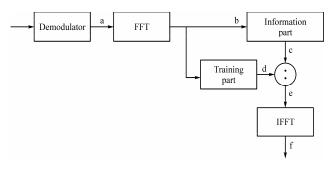
Fig. 3. Block diagram of the ISPR: FFT – fast Fourier transform, IFFT – inverse Fourier transform
