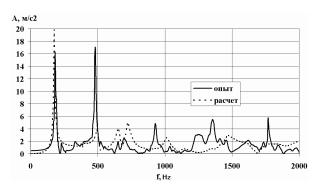
Fig. 6. Results of the design and experimental models' dynamic analysis
