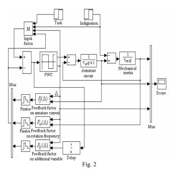
The block diagram of a model will consist of connected in series model PWC and parts of a control object of a direct current electric drive system, where q is a dimensionless Laplace operator. The variable factors of feedback dependent on value  $\Delta$  given out by the PWC which are switched *N* times for IP are included in models. Relative constants of time  $\tau_a$  u  $\tau_m$  are *N* times less than  $\theta_a$  and  $\theta_m$  [4].
