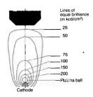
Fig. 2. Brightness distribution in the XBO-lamp arc
