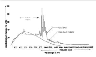
Fig. 3. Spectral radiation rate of the XBO-lamp
