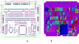
Fig. 4. General view of the unit with PCB and EEE parts (*a*); unit plate with automatically generated EEE parts' mass simulators (*b*)
