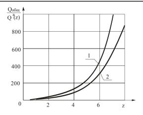
Fig. 6. The dependence of breakdown relation probabilities for the initial system and the breakdown probability of the system, divided into z parts and calculated according to the alternative technique from z, with n = 16, m = 2;
