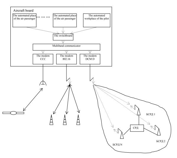
Fig. 7. The offered HSWTI structure for aeronautics telecommunication
