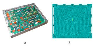
Fig. 2. Appearance of the onboard unit (*a*); detailed FEM of its frame (*b*)
