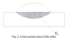
It is established that fusion penetration of the parent metal is minimal; the share of the parent metal in surfaced one has reached 10 %. It is obvious, that the method of
