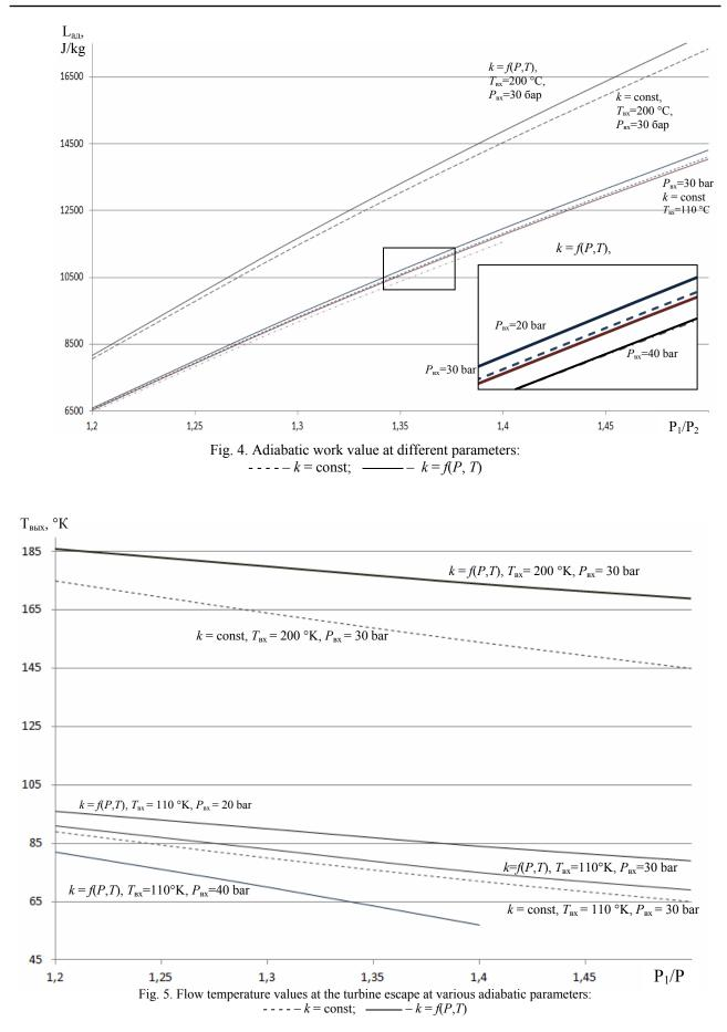
The given calculations show that the registering of the adiabatic curve indications is necessary for more accurate determination of the thermodynamic parameters for the compressor and turbine performance. The calculation of the kinematic parameters of the flow in the system and the design of the flow sector and turbine or compressor blades should also be carried out taking into account the variability of the adiabatic curve indicator.
