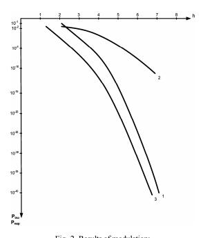
Fig. 2. Results of modulation: 1 – the probability of pairwise transition of one invariant into another under the following given conditions: k = 1;  $INV_1 = 1$ ;  $INV_2 = 2, 3, ..., 6$  and non-coherent reception; 2 – the probability of error in classical amplitude modulation and non-coherent reception; 3 – the probability of the pairwise transition of one invariant into another under the following given conditions: k = 1;  $INV_1 = 1$ ;  $INV_2 = 2, 3, ..., 11$  and coherent reception
