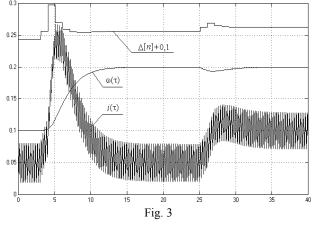
As it has already been mentioned the actual size of pure delay can vary rather widely and under its significant deviation from the calculated value transients can be completely unacceptable. The developed technique of modal regulators synthesis allows to exclude subharmonic oscillations typical for high-speed systems with a part of pure delay in the control channel. Subharmonic
