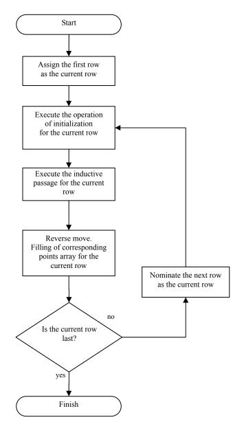
Fig. 3. The dynamic programming algorithm
