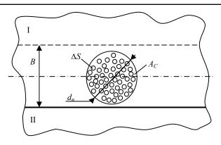
Fig. 3. Model of sieve contact conductivity
