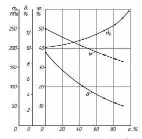
Fig. 6. Changing of mechanical properties of semi-finished items made of alloy AJ31 chips after hot pressing  $(\varepsilon = 0 \%)$  and cold drawing
