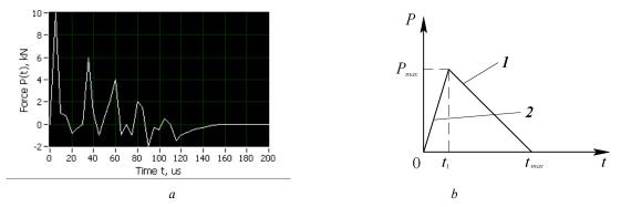
Fig. 4. The contact force time function P(t)(a) and pulse envelope (b) at transversal central impact on the firmly fixed glass fiber plate:  $1 - P = P_{max} (1 - t/t_{max}); 2 - P = P_{max} t/t_1$
