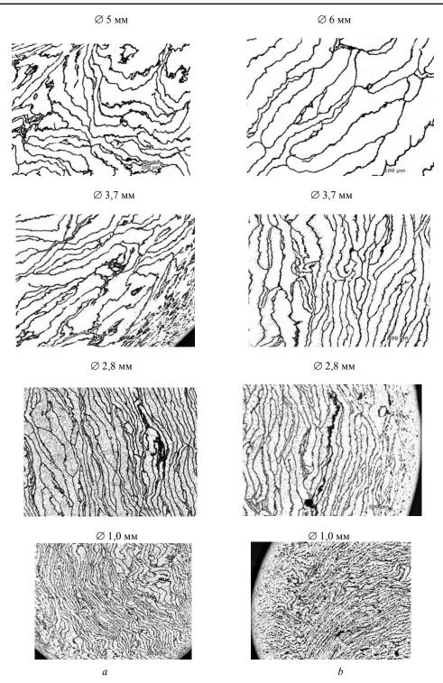
Fig. 5. The cross-sectional microstructure of the wire made in different compression modes from rods with diameters of 7 (a) and 9 (b) mm
