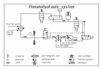
Fig. 1. Pneumohydraulic system using helicopter oil system as a source of heat
