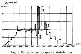
Fig. 1. Radiative energy spectral distribution of the ДКсРМ-55000-УХЛ-4 lamp
