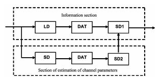
Fig. 1. Extended structural scheme of an invariant system: LD is a linear detector; DAT is a digital – analogue transducer; SD1 is a solving device 1; SD is a synchronous detector; SD2 is a solving device 2
