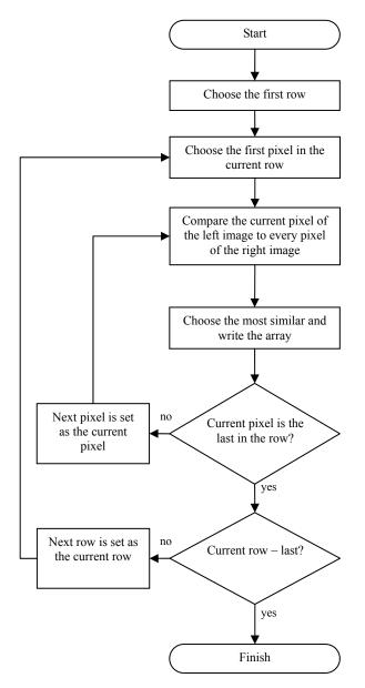
Fig. 1. The logical diagram of the stereovision functioning for a simple algorithm
