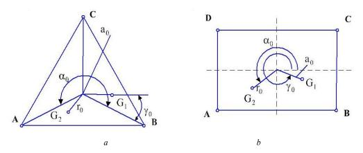
Fig. 1. The general analytical models to determine support reaction for multi-support contours: A, B, C, D are contour determining points;  $a_0$  is an angle of displacement from a central point;  $r_0$  is a displacement radius of a center of mass;  $G_1$   $\mu G_2$  are gravities;  $\gamma_0$  is a constant angular displacement of a fixed part center of mass relative to a geometric support contour center
