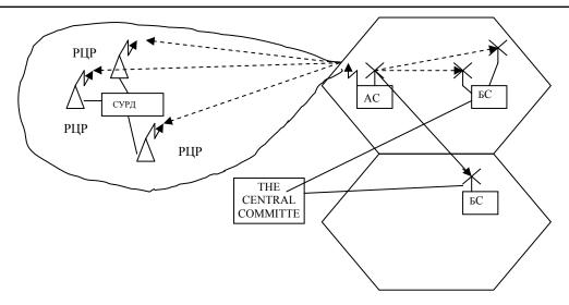
Fig. 1. Ways of spacious separation for signal reception in hybrid networks of wireless information transfer
