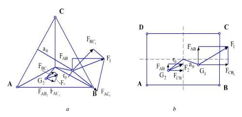
Fig. 2. The general analytical models to determine support reaction for four-support contours: A, B, C, D are points determining the contour;  $a_0$  is the angle of displacement from a central point;  $r_0$  is a displacement radius of a center of mass;  $G_1
