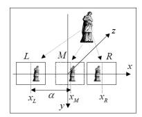
Fig. 2. Geometry of stereo filming
