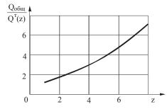
Fig. 5. The dependence of relation for the common reserving initial system breakdown probability and the breakdown probability of the system, divided into *z* parts from *z*, applying
