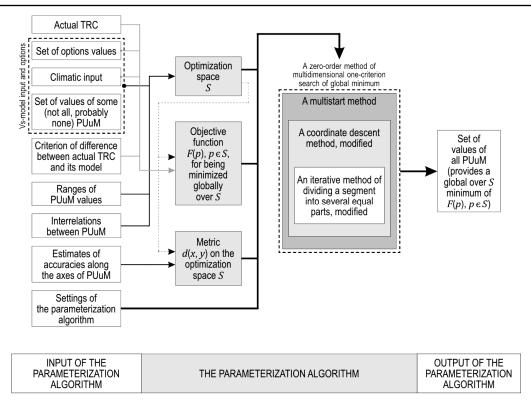
Structural scheme of the parameterization algorithm for the VS-model
