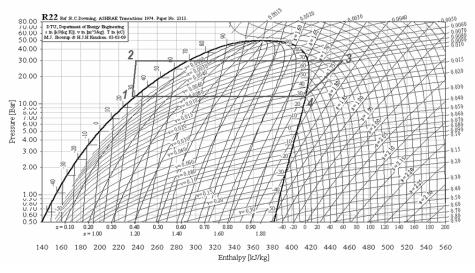
Fig. 2. Plant cycle in *lg P–I* coordinates
