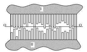
Fig. 1. Contact of two rough surfaces. The rod model
