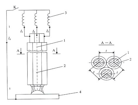
Fig. 1. Scheme of surfacing by indirect three-phase arc:
