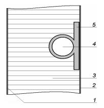
Fig. 1. Fragment of a honeycomb panel with a heat pipe
