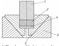
Fig. 1. The scheme of the briquette making mold for combined rolling and pressing
