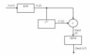
Fig. 4. Structure of the IFOTS receiving part
