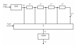
Fig. 2. The structure of the signal shaper for the N = 4 IFOTS
