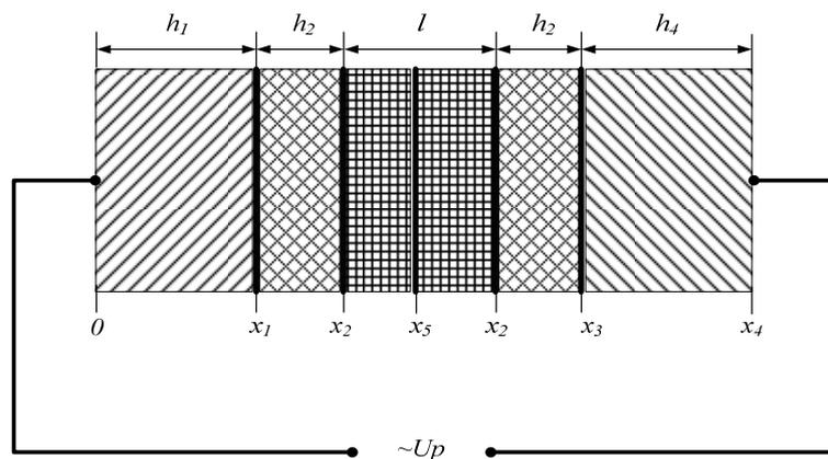
Fig. 5. Appliance for high-frequency processing of parts:
