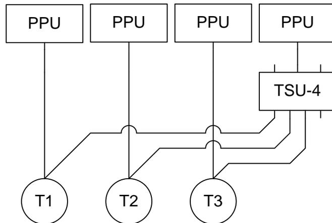
Fig. 13. Constant powering of three out of three thrusters with PPU reservation
