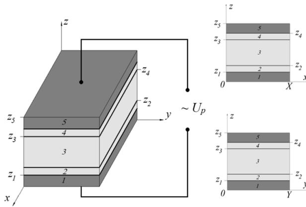
Fig. 8. 3D five-layer high-frequency processing technological scheme.
