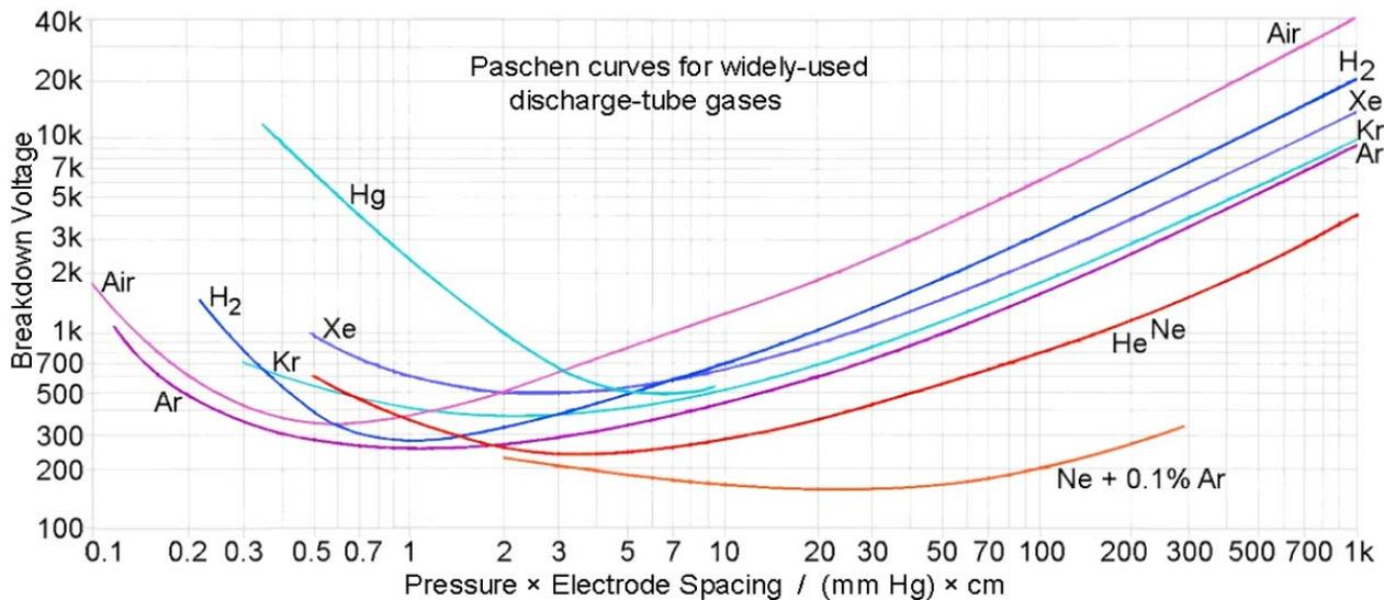
Fig. 2. Paschen curves for different gases
