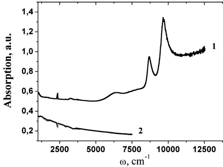
Fig. 4. Optical absorption spectra for  $MnSe_{1-x}Te_x$  solid solutions with  $X = 0.2$  (1),  $0.4$  (2) at  $T = 300$  K
