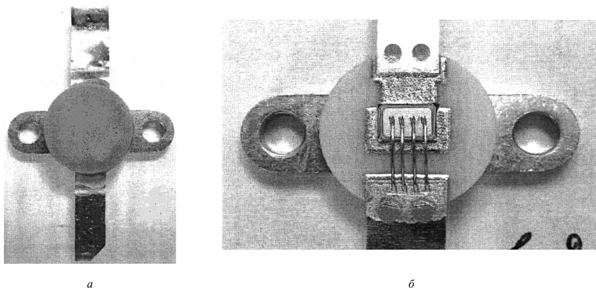
Fig.1. Standard hermetic EEE housing design:
