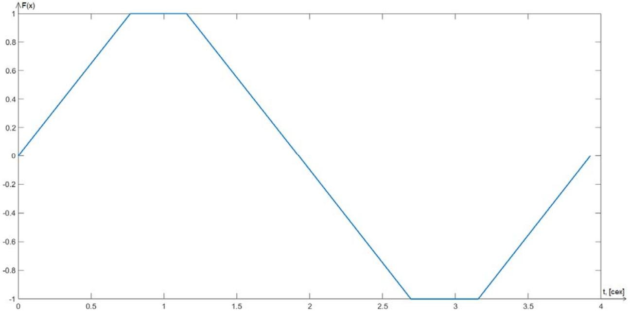
Fig. 6. The shape of the controlling signal in the form of a triangle with saturation zones
