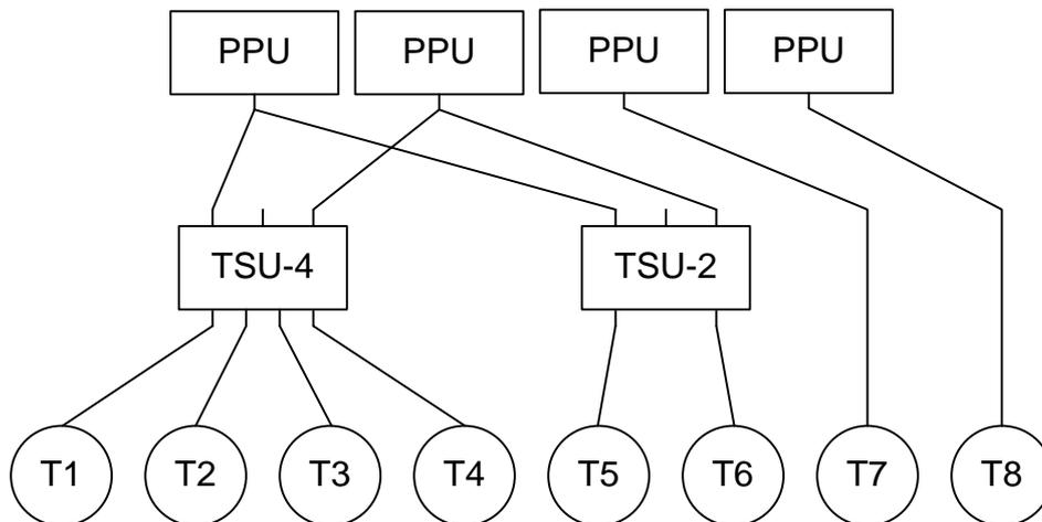
Fig. 11. Temporary powering of four out of eight thrusters and constant powering of one out of four thrusters
