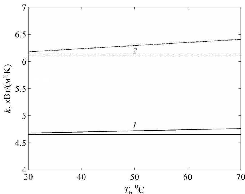
Fig. 5. Dependence of the heat transfer coefficient on the wall base temperature
