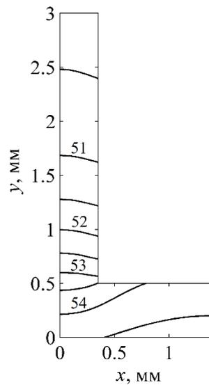
Fig. 4. Temperature field of the finned wall with the thickness of the fin 0.7 mm and the wall 0.5 mm
