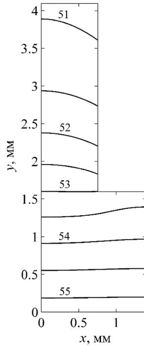
Fig. 3. Temperature field of the finned wall with the thickness of the fin 1.5 mm and the wall 1.6 mm
