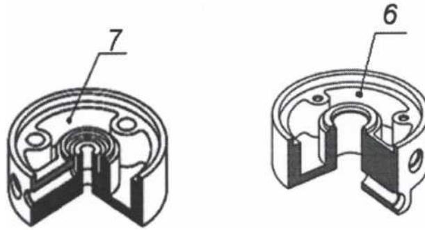
Fig. 2. Cathode and anode assemblies
