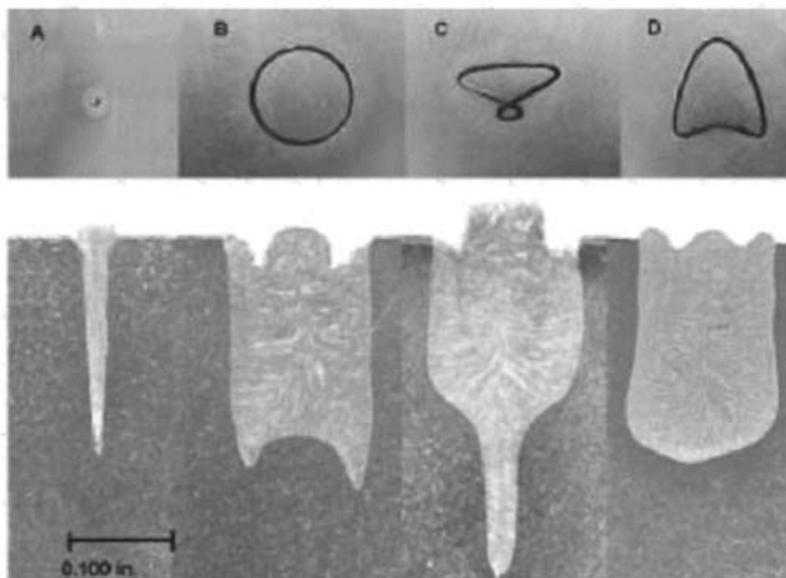
Fig. 1. Influence of the beam scanning trajectory on the weld cross-section:
