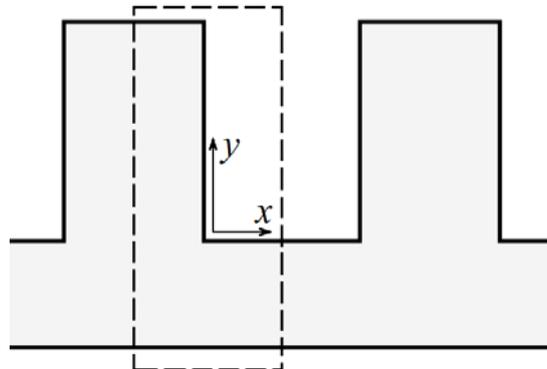
Fig. 1. Diagram of the finned wall and the boundary of the calculation area
