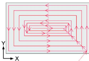
Fig. 2. New trajectories for melting a rectangular area
