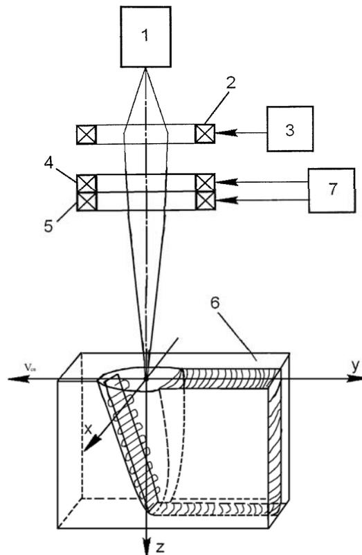
Fig. 3. A scheme of electron-beam welding when scanning in the form of a raster:
