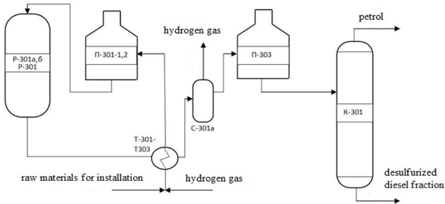
Fig. 4. Fragment of a scheme for hydrotreating diesel fuel and hydrodewaxing
