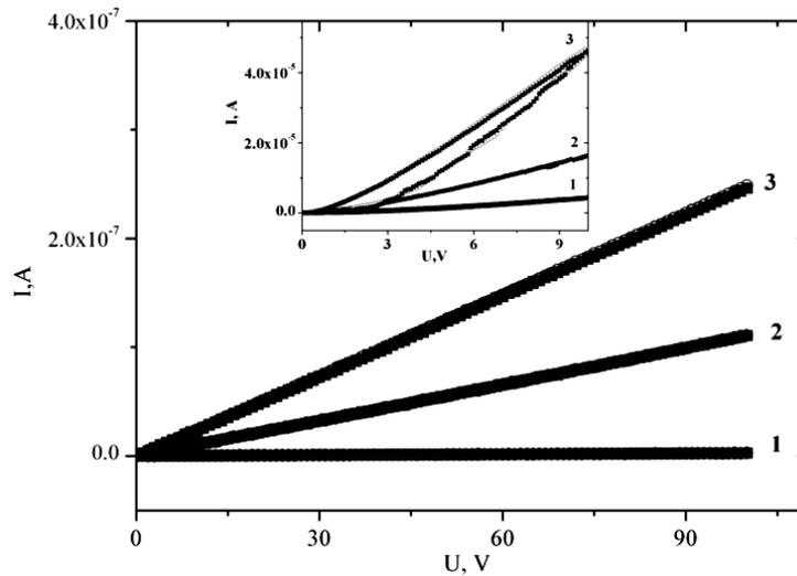
Fig. 6. The current-voltage characteristics measured in a zero magnetic field (empty circles) and field 12 kOe (black circles). MnSe<sub>0.9</sub>Te<sub>0.1</sub> at  $T = 80$  K(1), 180 K(2) and 220 K(3).
