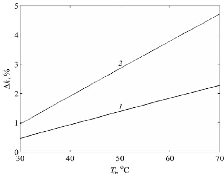
Fig. 6. Relative error in calculating the heat transfer coefficient in a simplified approximation
