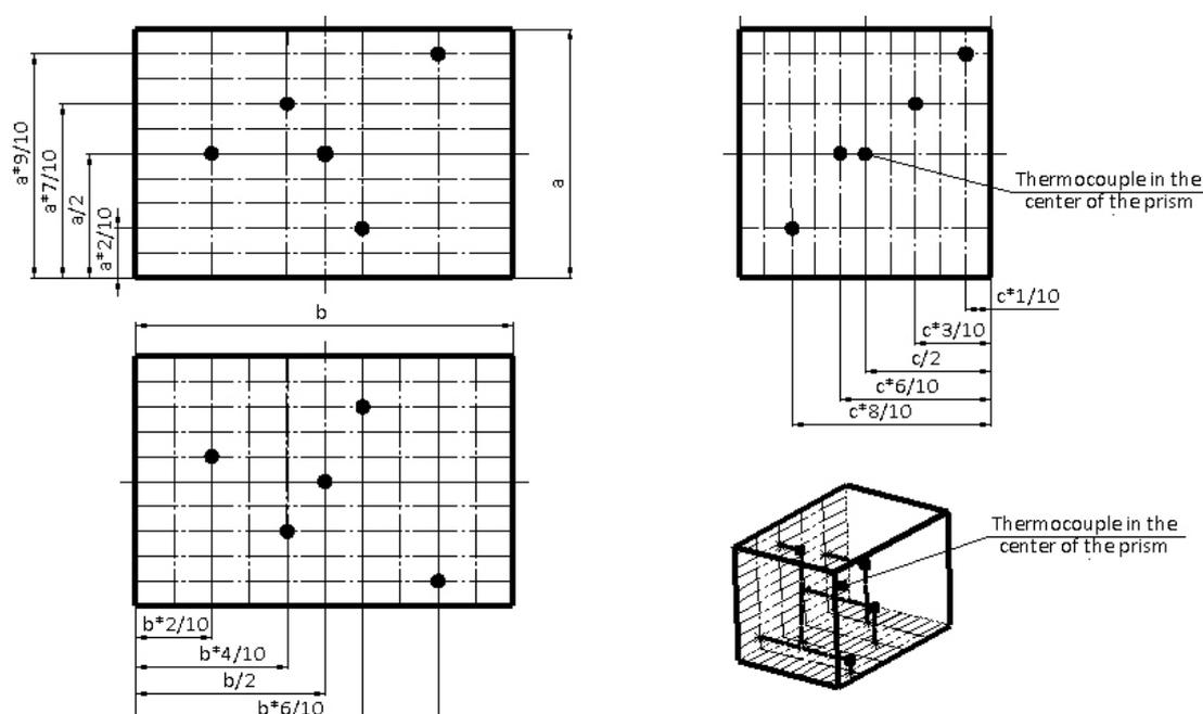
Fig. 1. Layout of thermocouples in the sample
