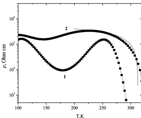
Fig. 5. The temperature dependence of the electrical resistivity for films  $\text{MnSe}_{0.9}\text{Te}_{0.1}$  (1) and  $\text{MnSe}_{0.8}\text{Te}_{0.2}$  (2). The dotted line indicates that the temperature dependence of the resistance is described by a power function (6)
