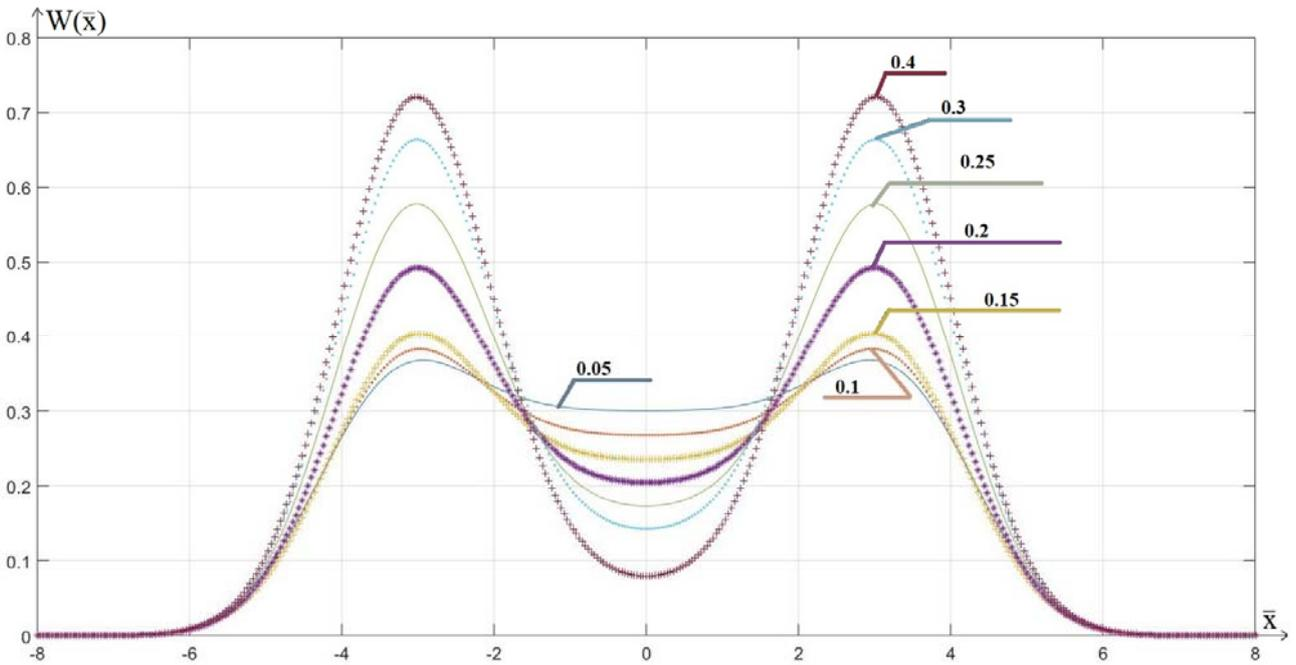
Fig. 7. Beam energy distribution on the surface of a detail when scanning with a truncated raster and changing the boundaries of the saturation zone
