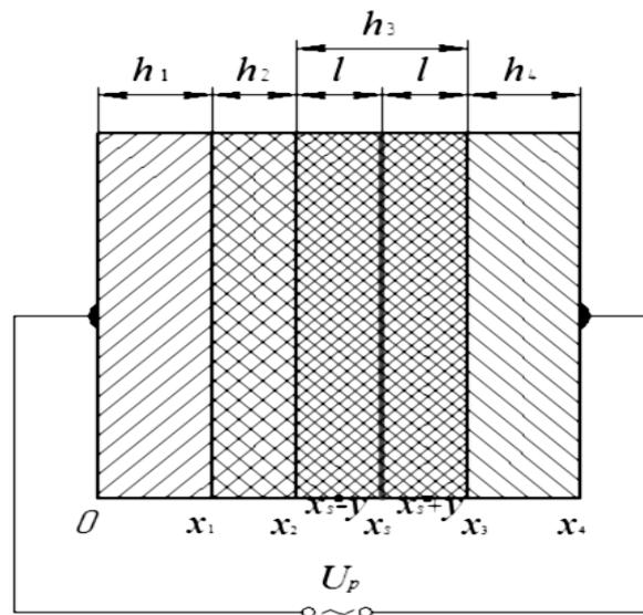
Fig. 3. High-frequency welding of plastic parts in industrial equipment with one insulated electrode, where  $h_1, h_4$  is the thickness of the high potential and grounded electrodes;  $h_2$  is the thickness of the insulating liner;  $l = h_3/2$  – thickness of the welded part;  $x_i$  is the coordinate of the layer boundary;  $x_s$  is the coordinate of the weld;  $y$  is the distance from the weld;  $U_p$  is the voltage at the working capacitor
