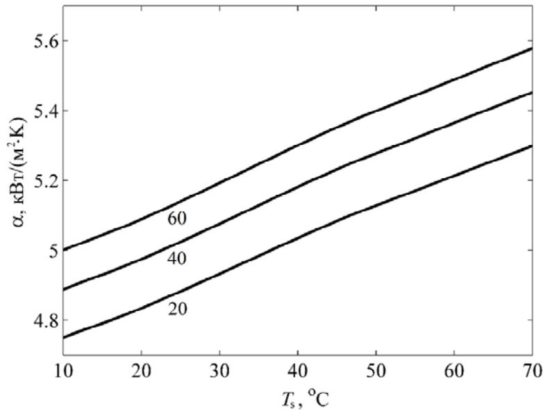
Fig. 1. Dependence of the local heat transfer coefficient LZ-TK-2 on the wall temperature
