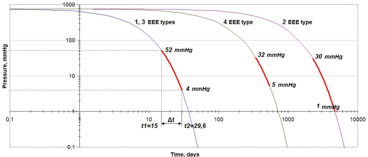
Fig. 3. Graph of pressure drop at the rate of hermeticity index for TS with indication of the Paschen zone for each type of EEE (pressure, mmHg; types of EEE; time, full day)
