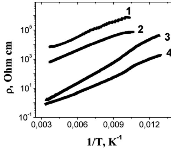
Fig. 1. Temperature dependence of the electrical resistivity  $\text{MnSe}_{1-X}\text{Te}_X$  solutions with concentration of  $X=0.1$  (1), 0.2 (2), 0.3 (3), 0.4 (b)
