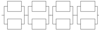
Fig. 4. The essential system, divided into  $z = 4$  parts and transformed into the individual reserving scheme
