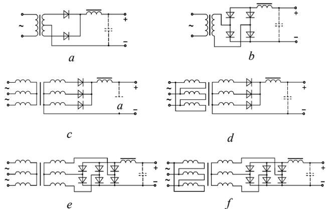
Fig. 2. Rectifiers operating at inductance;
