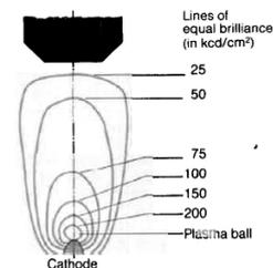
Fig. 2. Brightness distribution in the XBO-lamp arc
