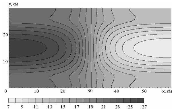
Fig. 3. Temperature field of a honeycomb panel external surface
