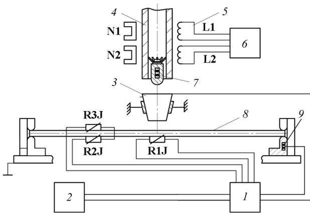
Fig. 1. The scheme of the automated test stand to study beams and plates non-stationary deformation processes under lateral shock loading:
