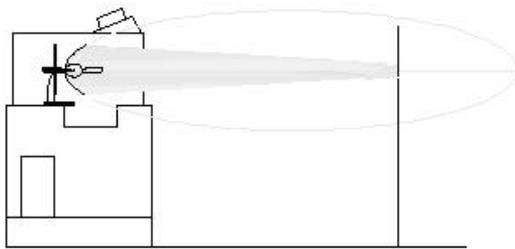
Fig. 4. The scheme of the experimental test bench for verification of XBO 10000 W/HS OFR lamp performance
