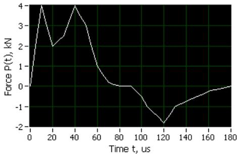
Fig. 3. Contact force time function  $P(t)$  at transverse central impact on the glass fiber hinged beam
