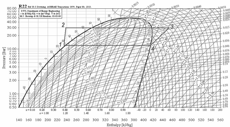
Fig. 2. Plant cycle in  $lg P-I$  coordinates
