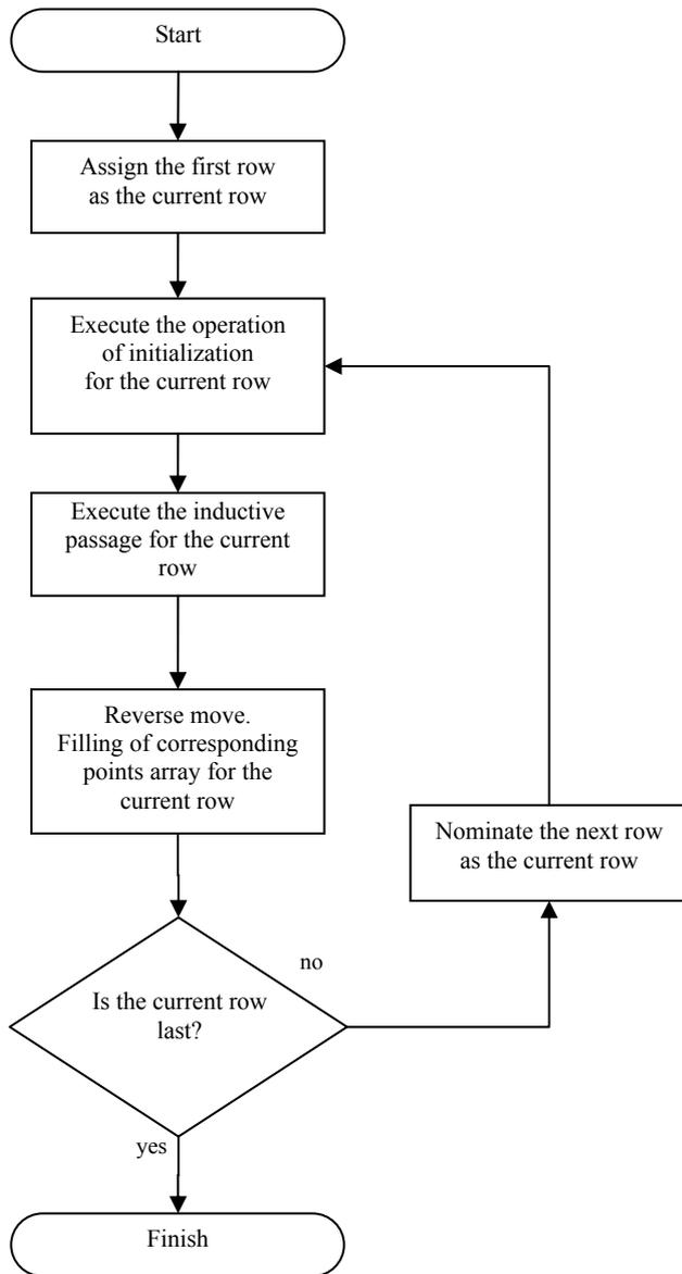
Fig. 3. The dynamic programming algorithm
