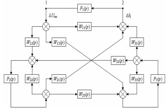
Fig. 1. Three-loop structural representation of EPS
