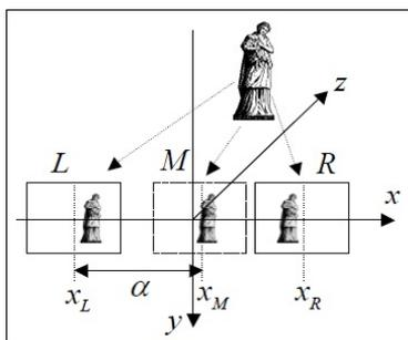
Fig. 2. Geometry of stereo filming
