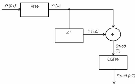
Fig. 4. Structure of the IFOTS receiving part
