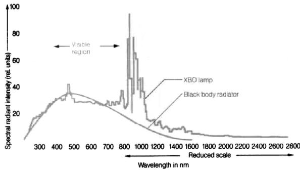
Fig. 3. Spectral radiation rate of the XBO-lamp
