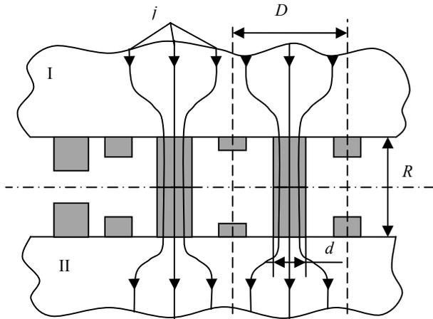
Fig. 2. Contact conductivity in the rod model
