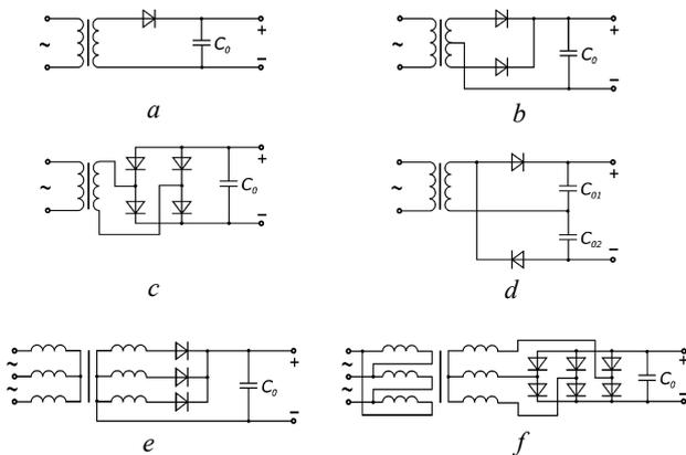
Fig. 1. Rectifiers operating at capacity:
