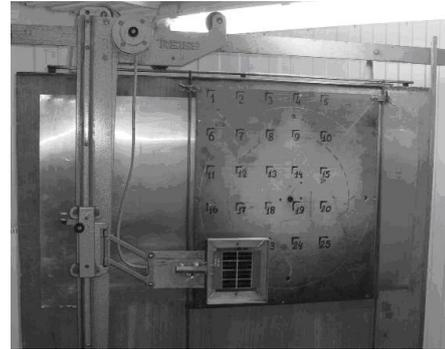
Fig. 6. The screen with marks for flux density scanning
