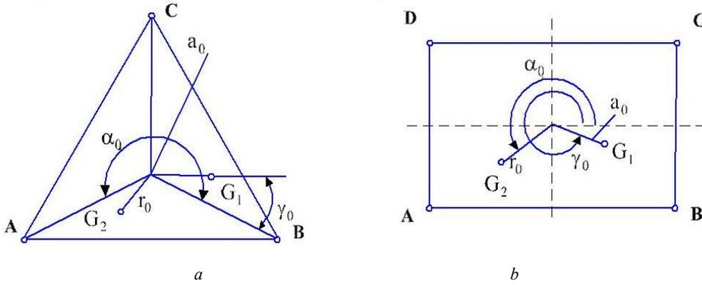
Fig. 1. The general analytical models to determine support reaction for multi-support contours:  $A, B, C, D$  are contour determining points;  $a_0$  is an angle of displacement from a central point;  $r_0$  is a displacement radius of a center of mass;  $G_1$  и  $G_2$  are gravities;  $\gamma_0$  is a constant angular displacement of a fixed part center of mass relative to a geometric support contour center
