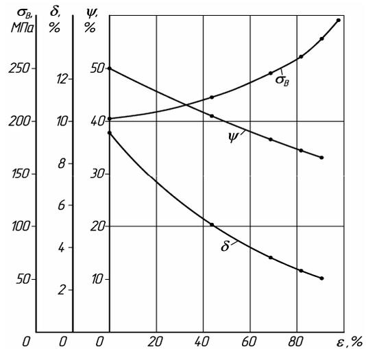
Fig. 6. Changing of mechanical properties of semi-finished items made of alloy AD31 chips after hot pressing ( $\varepsilon = 0\%$ ) and cold drawing
