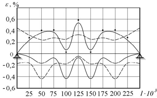
Fig. 5. Maximal bay bending  $\varepsilon_b$  (solid) and shear  $\varepsilon_s$  (dashed) strains of the hinged beam loaded by the transversal central sine pulse: lines stand for calculation data; points stand for experimental data
