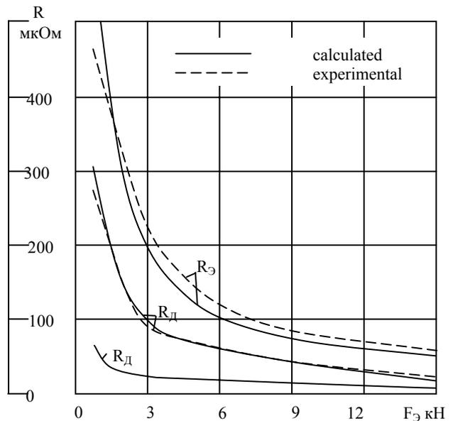
Fig. 4. Results of experimental and calculated resistance values
