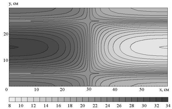
Fig. 2. Temperature field of a honeycomb panel internal surface
