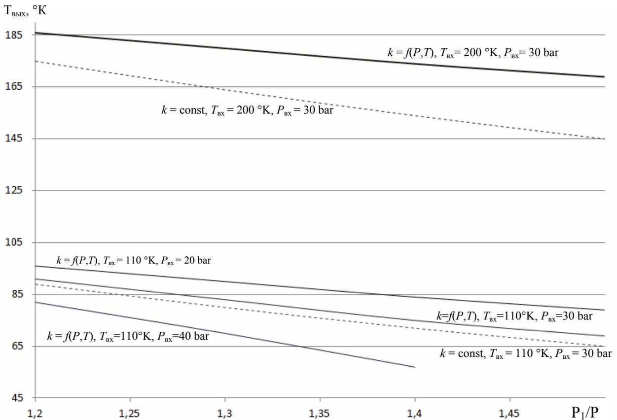
Fig. 5. Flow temperature values at the turbine escape at various adiabatic parameters:
