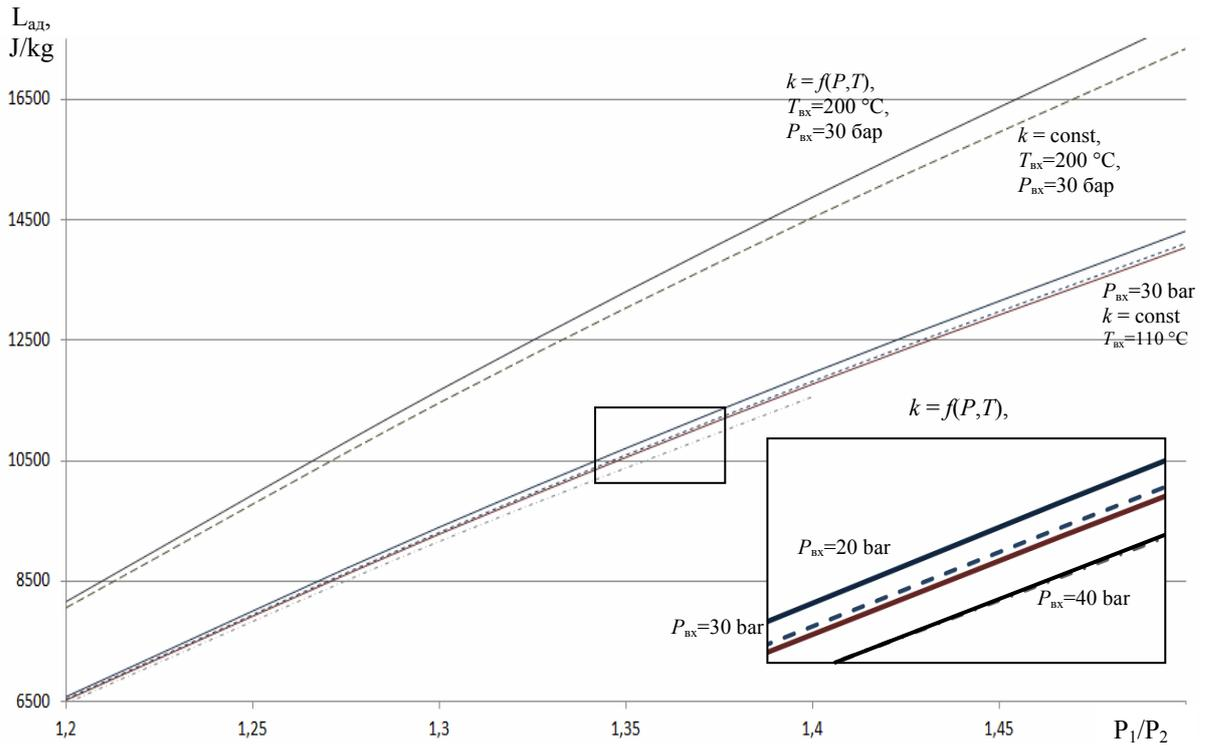
Fig. 4. Adiabatic work value at different parameters:
