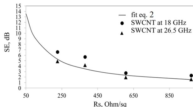
Fig. 6. Shielding efficiency as a function of sheet resistance for SWCNT films at the boundaries of the studied range
