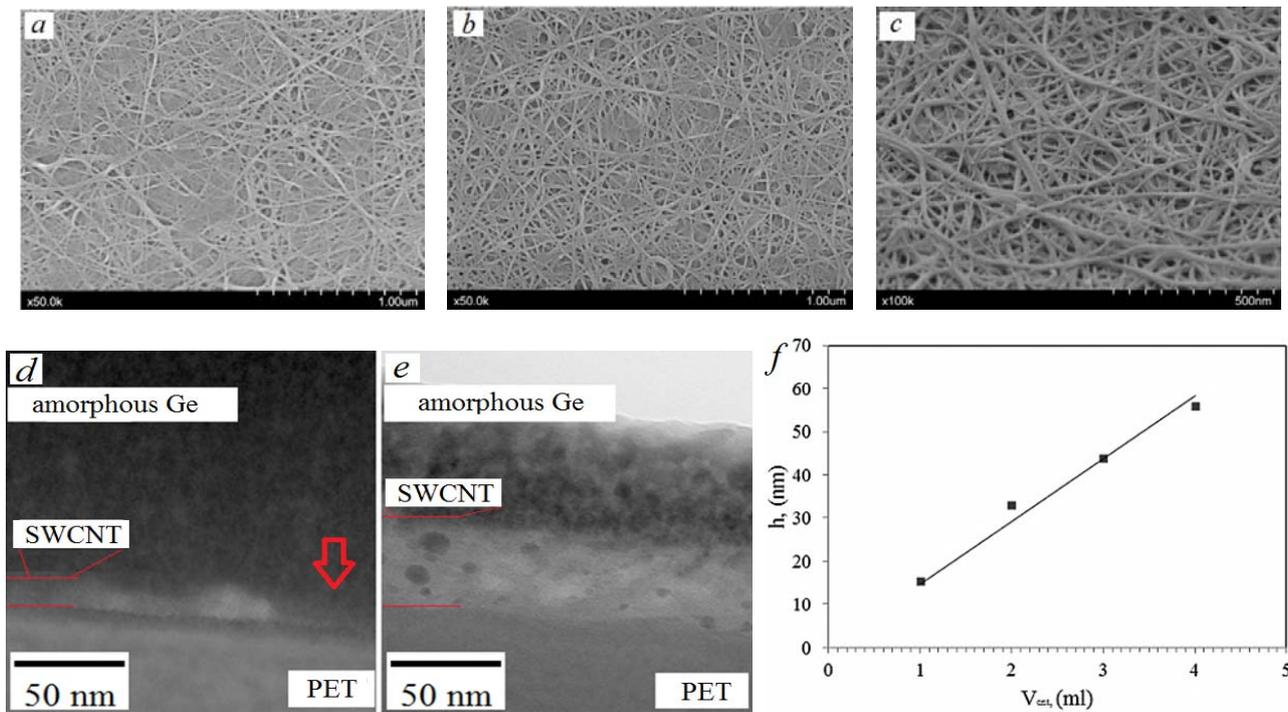
Fig. 1. SEM images of SWCNT films of various thicknesses: 1 ml (*a*) and 3 ml (*b* and *c*) of dispersion; TEM image of SWCNT films of various thicknesses: 1 ml (*d*) and 3 ml (*e*) of dispersion. Dependence of the SWCNT films thickness on the volume of sprayed dispersion (*f*)
