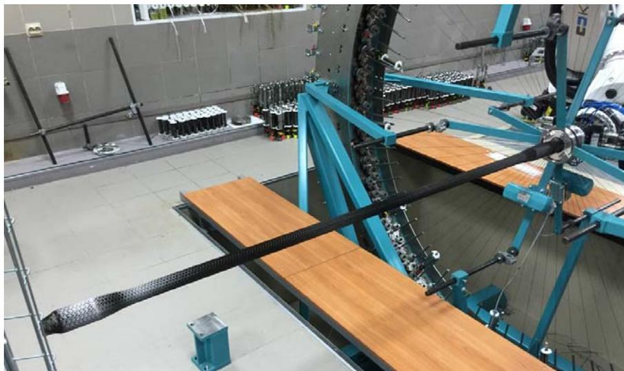
Fig. 2. Process of radial braiding of a tubular structure
