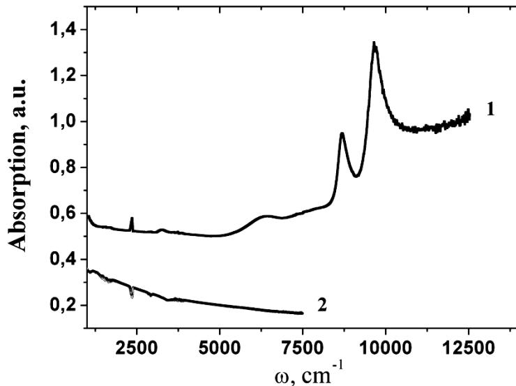
Fig. 4. Optical absorption spectra for  $\text{MnSe}_{1-X}\text{Te}_X$  solid solutions with  $X = 0.2$  (1),  $0.4$  (2) at  $T = 300$  K
