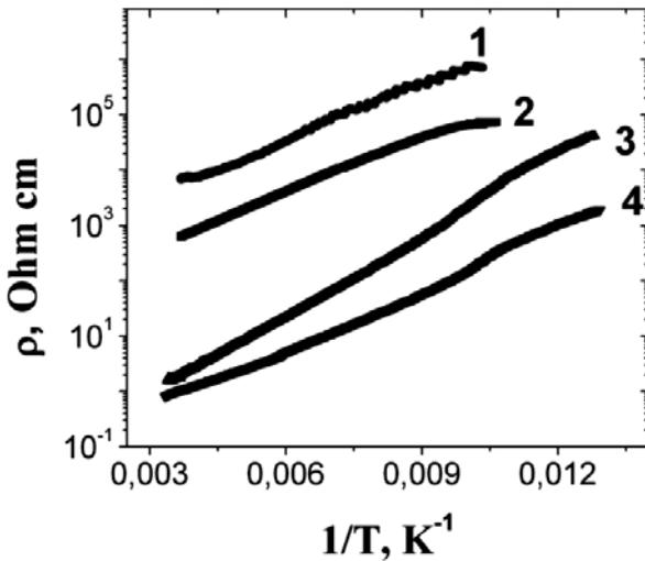
Fig. 1. Temperature dependence of the electrical resistivity  $\text{MnSe}_{1-X}\text{Te}_X$  solutions with concentration of  $X = 0.1$  (1), 0.2 (2), 0.3 (3), 0.4 (4)
