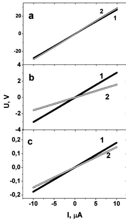
Fig. 2. The current-voltage characteristic of the  $\text{MnSe}_{1-X}\text{Te}_X$  solid solution ( $X = 0.1$ ) in a magnetic field  $H = 1$  T (2) and in a zero magnetic field (1) at different temperatures  $T$ : 100 K (a), 140 K (b), 190 K (c)
