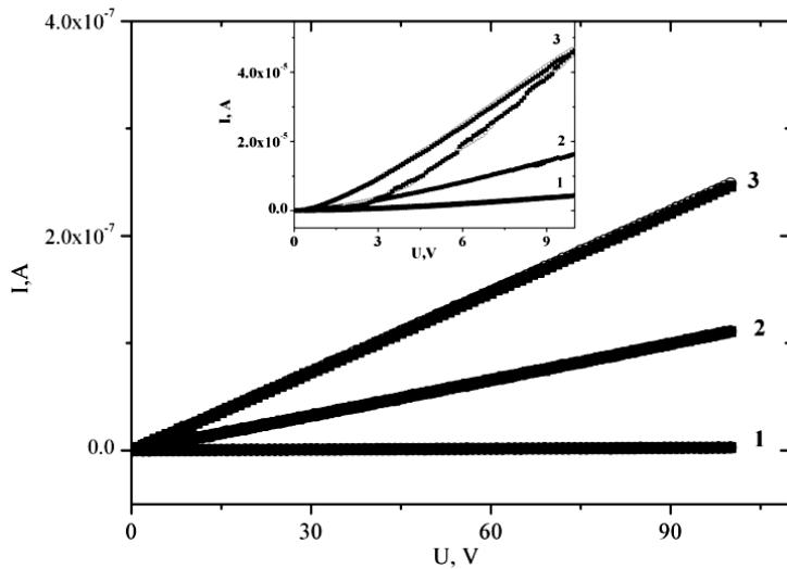
Fig. 6. The current-voltage characteristics measured in a zero magnetic field (empty circles) and field 12 kOe (black circles). MnSe<sub>0.9</sub>Te<sub>0.1</sub> at  $T = 80$  K(1),  $180$  K(2) and  $220$  K(3).
